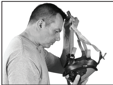
FIGURE 11-B HARNESS OUT OF WAY
